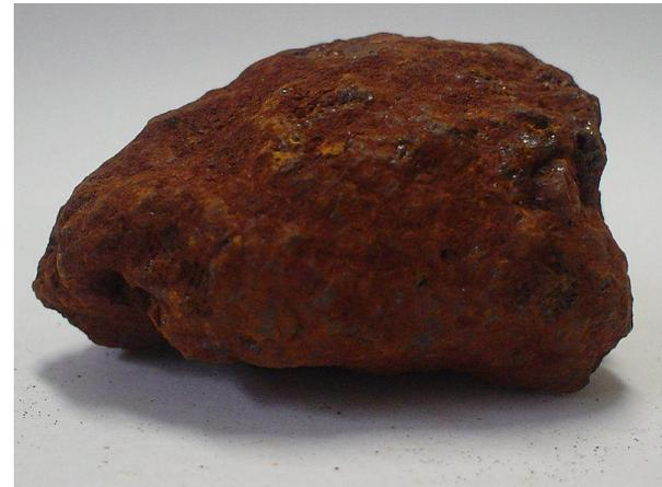
Hematita ( $\text{Fe}_2\text{O}_3$ )
