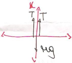
$$\bullet \Sigma F_y = T + T - mg = 0 \quad (\text{no se mueve})$$
