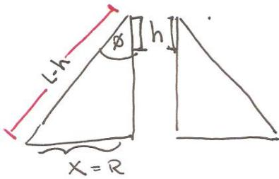
$$\begin{aligned} \bullet \sin\phi &= \frac{x}{L-h} \\ \Rightarrow \boxed{x = (L-h)\sin\phi} &= R \end{aligned}$$
