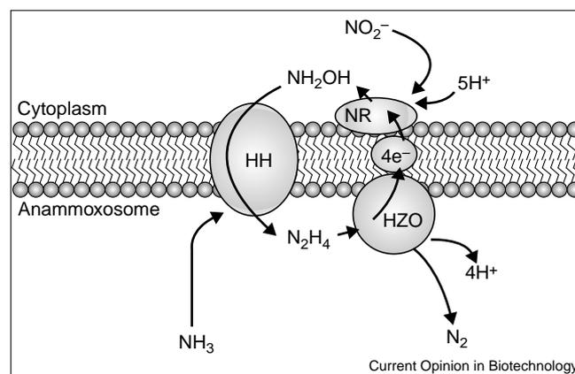
Mechanism of anaerobic ammonium oxidation. NR is a nitrite-reducing enzyme ( $\text{NH}_2\text{OH}$  is the assumed product); HH (hydrazine hydrolase) condenses hydrazine out of ammonia and hydroxylamine; HZO is a hydrazine-oxidising enzyme (which might be equivalent to hydroxylamine oxidoreductase).
