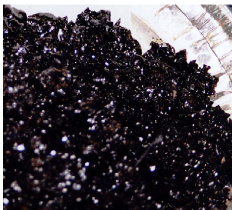
Fig. 4. EFSb-FC slag sample after re-melting and fast cooling.
