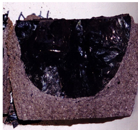
Fig. 3. EFSa-SC slag sample after re-melting and slow cooling.
