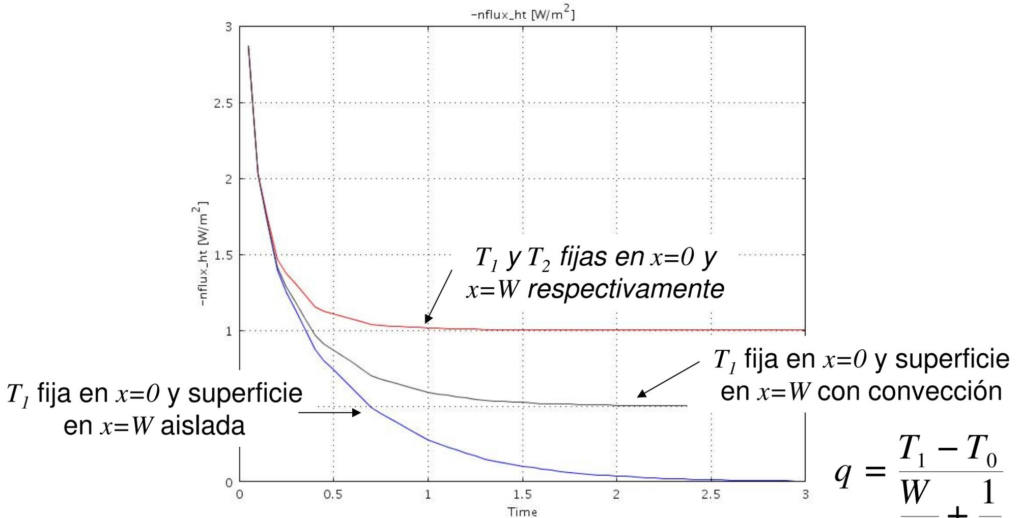
$$q = \frac{T_1 - T_0}{\frac{W}{k} + \frac{1}{h}}$$
