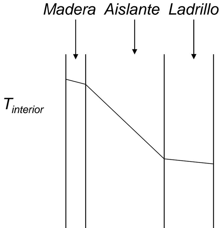
$$\left[ \frac{dT}{dx} \right]_{madera} = \frac{k_{ladrillo}}{k_{madera}} \left[ \frac{dT}{dx} \right]_{ladrillo} = 4.7 \text{ } ^\circ\text{C}$$
