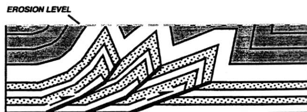
Figure 4.2.3. Blind thrust system formed by a buried imbricate fan in which the overlying strata are shortened by folding.
