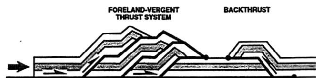
Figure 4.2.2. Backthrust showing an opposite sense of vergence to that of the foreland vergent thrust system.
