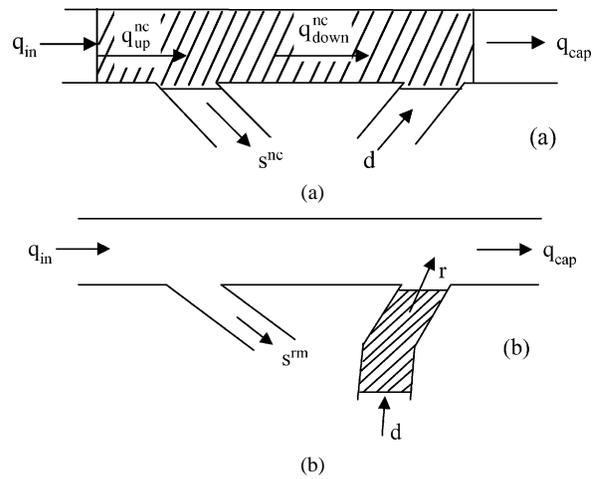
Fig. 3. Two cases: (a) without and (b) with ramp metering.
