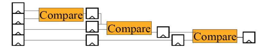
$$T_cp = t_ck-Q + t_logic + t_su + t_skew + t_jitter$$
