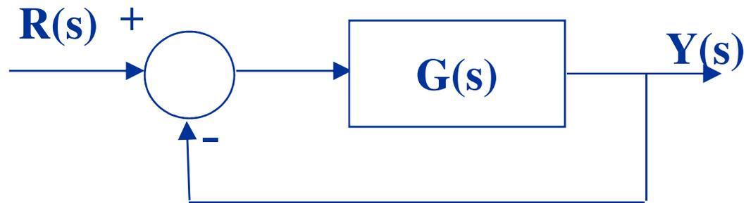
$$G(s) = \frac{K(T_a s + 1)(T_b s + 1) \cdots (T_n s + 1)}{s^N (T_1 s + 1)(T_2 s + 1) \cdots (T_p s + 1)}, \quad s^N : N \text{ polos en el origen}$$
