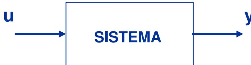
$$\left. \begin{array}{l} u_1 \Rightarrow y_1 \\ u_2 \Rightarrow y_2 \end{array} \right\} \begin{array}{l} u_1 + u_2 \Rightarrow y_1 + y_2 \\ K \cdot u_1 \Rightarrow K \cdot y_1 \end{array}$$
