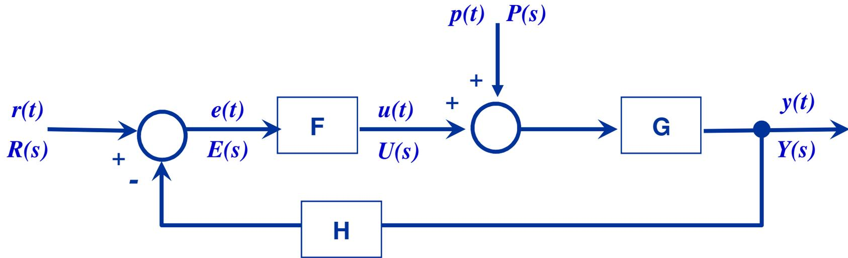
$$\left. \begin{aligned} Y &= G(P + F(R - HY)) \\ [1 + FGH] \cdot Y &= GP + FGR \end{aligned} \right\} \Rightarrow Y = \frac{G}{1 + FGH} \cdot P + \frac{FG}{1 + FGH} \cdot R$$
