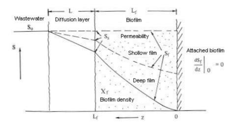
Simulate the removal of phenol from wastewater by biofilm. The governing equation can be formulated by Haldane equation at steady state is given by:
