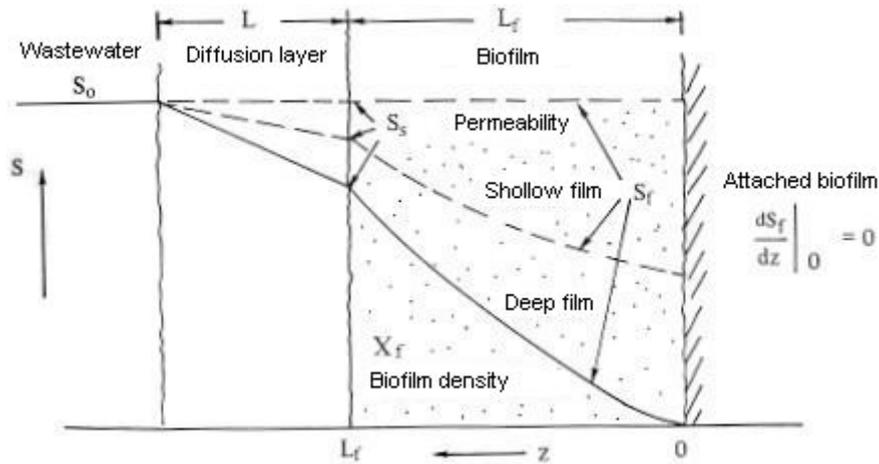
Simulate the removal of phenol from wastewater by biofilm. The governing equation can be formulated by Haldane equation at steady state is given by:
