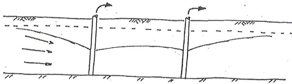
Flow is not horizontal - we use the Dupuit assumptions to develop the solution.
