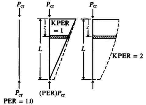
**Figure 16-25** Variation of  $P_{cr}$  with depth of embedment of the pile or pole. PER = computer program variable used by the author relating the assumed amount of  $P_{cr}$  at the point. KPER = computer variable to specify type of skin resistance reduction as shown.
