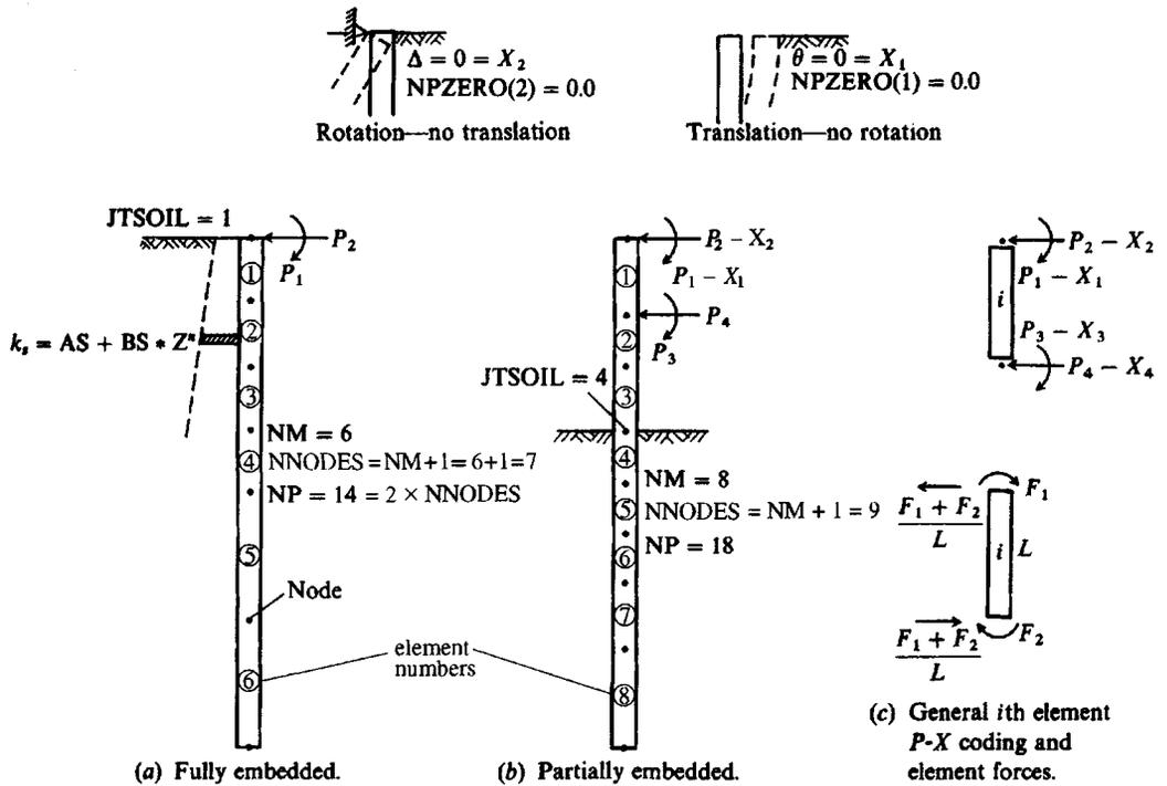
**Figure 16-19** Laterally loaded pile using finite elements. Typical loadings shown in (a) and (b). Note that elements do not have to be same size or length. Generally use short elements near ground surface and longer elements near pile point where moments are less critical.
