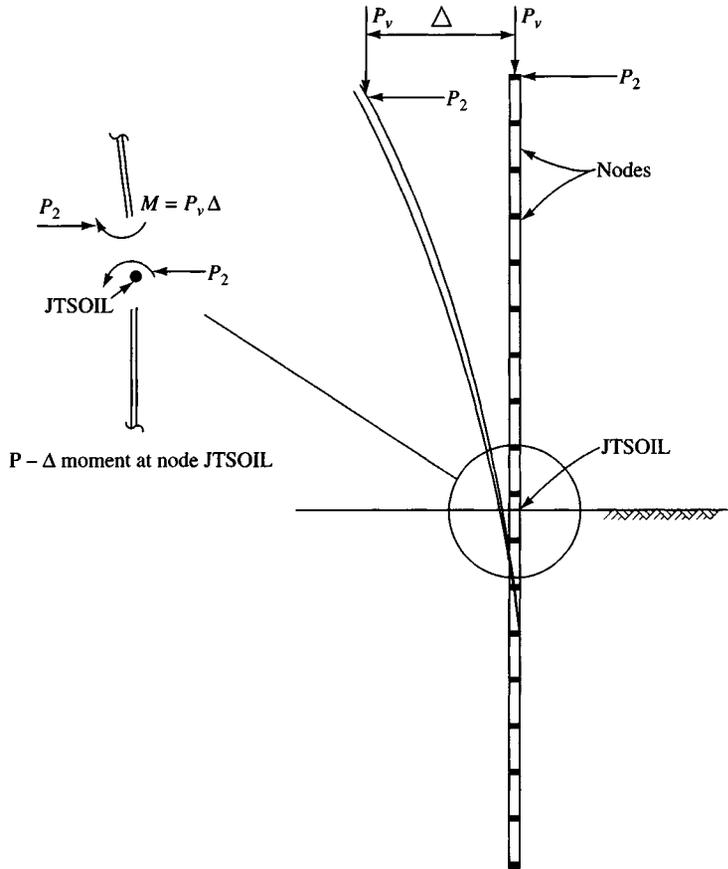
**Figure 16-21** The geometric  $P-\Delta$  effect for laterally loaded piles.
