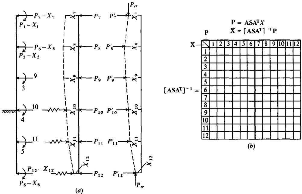
**Figure 16-23** (a) General coding and notation used in the pile-buckling problem. The ground line can be specified at any node. Develop the  $ASA^T$ , invert it, and obtain the  $D$  matrix from the location shown in (b).
