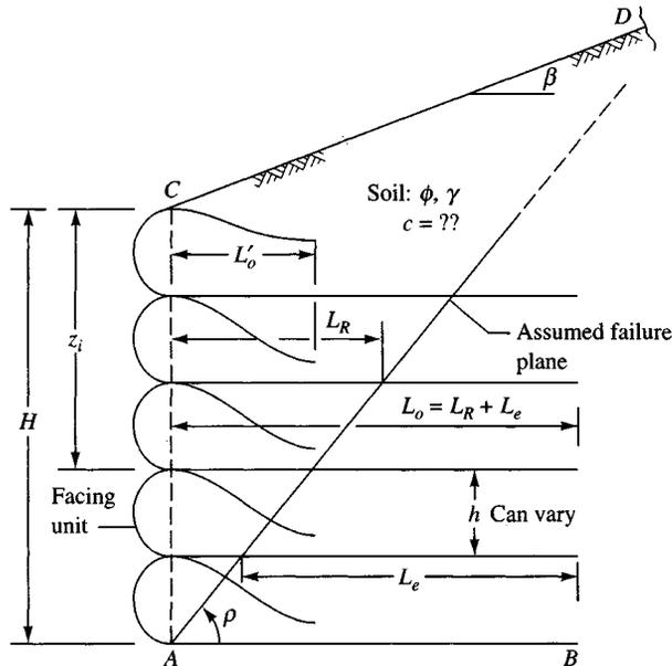
**Figure 12-3** Using geotextile sheets for reinforcement with the facing unit formed by lapping the sheet as shown. Critical dimensions are  $L_e$ ,  $L'_o$ , and  $L_o$ . Distances  $L_e$  and  $L_o$  are variable but for this wall produce a constant length  $L_{con} = L_o + L_e$ . The Rankine  $\rho \neq 45^\circ + \phi/2$  for backfill  $\beta$  as shown. Use your program SMTWEDGE (B-7) to find  $\rho$ , and make a scaled plot to check computed lengths.
