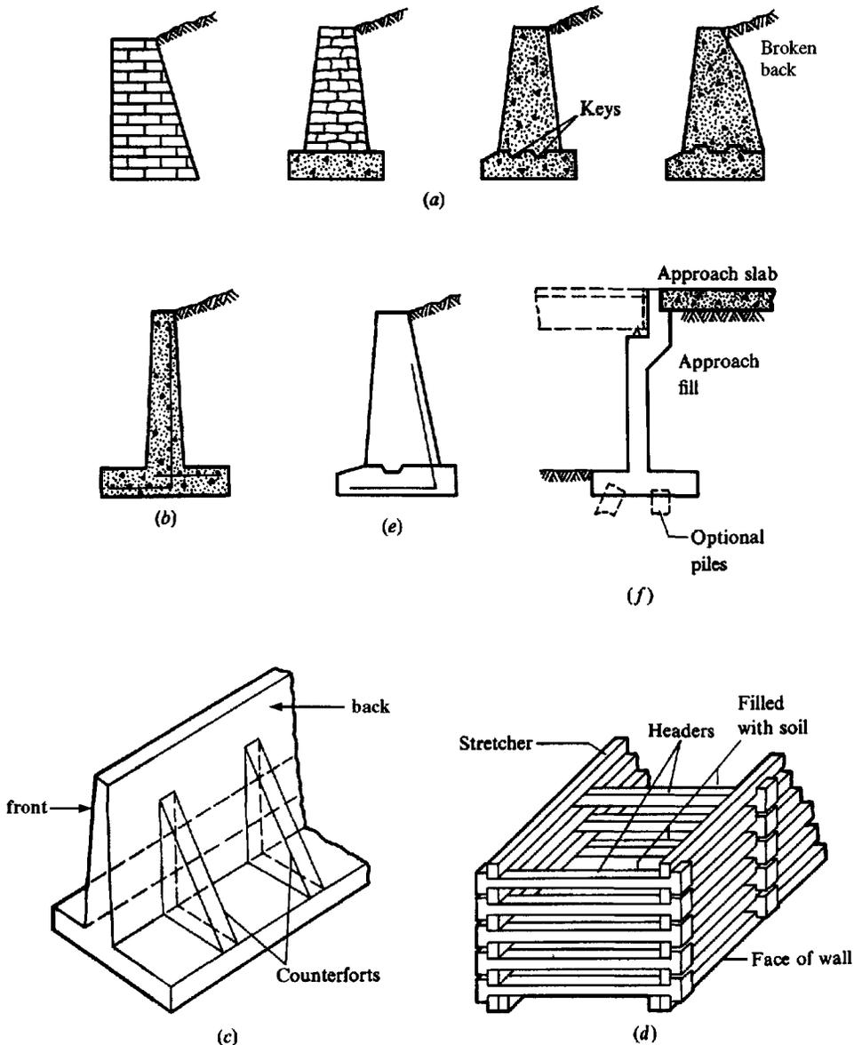
**Figure 12-9** Types of retaining walls. (a) Gravity walls of stone masonry, brick, or plain concrete—weight provides stability against overturning and sliding; (b) Cantilever wall; (c) Counterfort, or buttressed wall—if backfill covers the counterforts the wall is termed a counterfort; (d) Crib wall; (e) Semigravity wall (uses small amount of steel reinforcement); (f) Bridge abutment.
