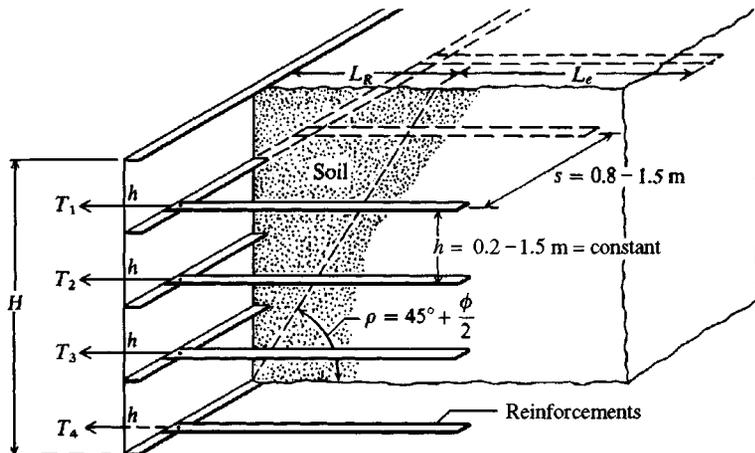
That is, the sum of the several tensile reinforcement forces should equal the lateral-earth-pressure diagram ratioed from a unit width to the actual reinforcement spacing  $s$ .
