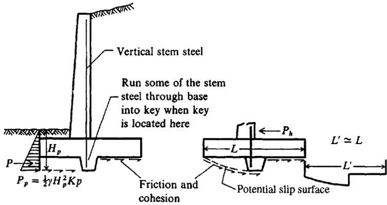
(a) Base key near stem so that stem steel may be extended into the key without additional splicing or using anchor bends. (b) Potential sliding surface using the key location of a. There may be little increase in sliding resistance from this key, if the slip surface develops as shown.
