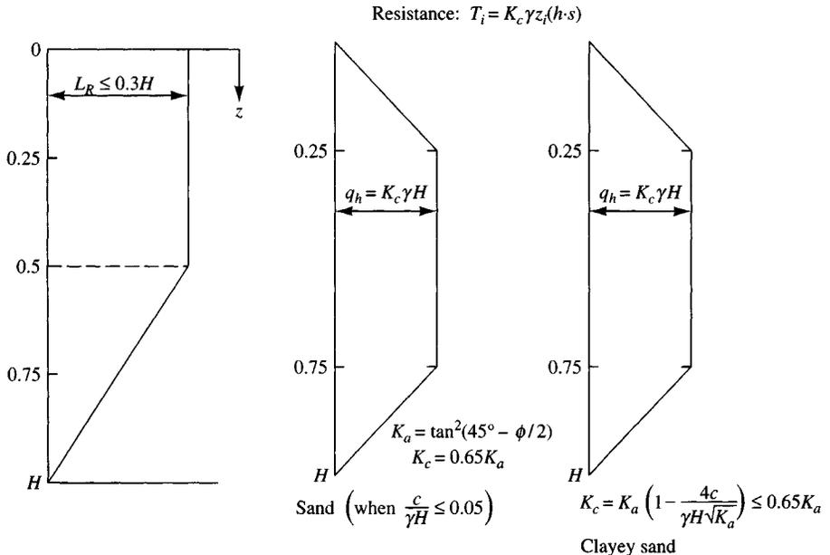
**Figure 12-8** Failure wedge and approximate pressure diagrams for soil nailing.
