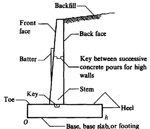
**Figure 12-10** Principal terms used with retaining walls. Note that “toe” refers to both point  $O$  and the distance from front face of stem; similarly “heel” is point  $h$  or distance from backface of stem to  $h$ .
