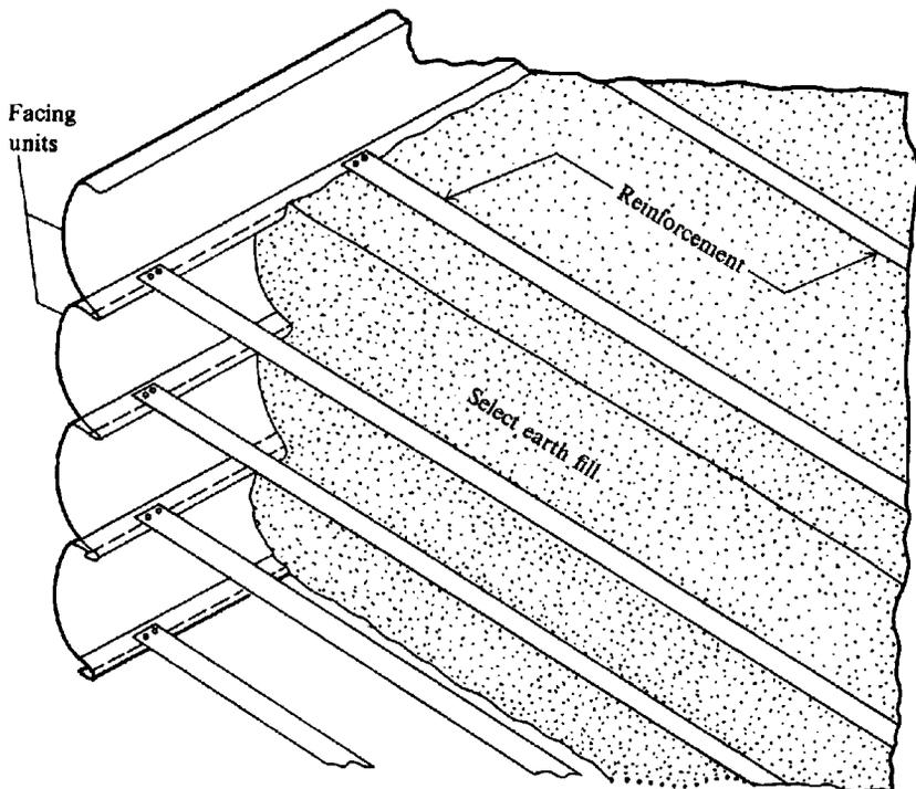
Figure 12-1 The reinforced earth concept. [After Vidal (1969).]
