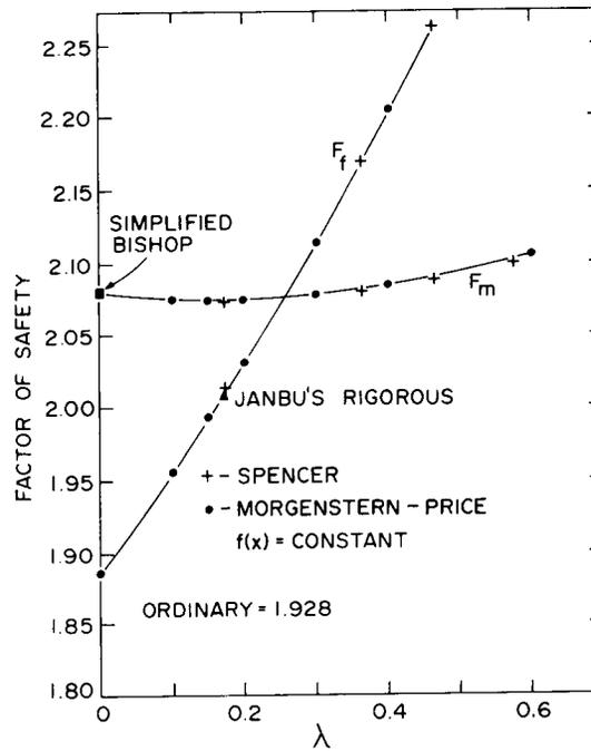
FIG. 9. Comparison of factors of safety for case 1.
