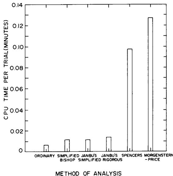
FIG. 13. Time per stability analysis trial for all methods of analysis.
