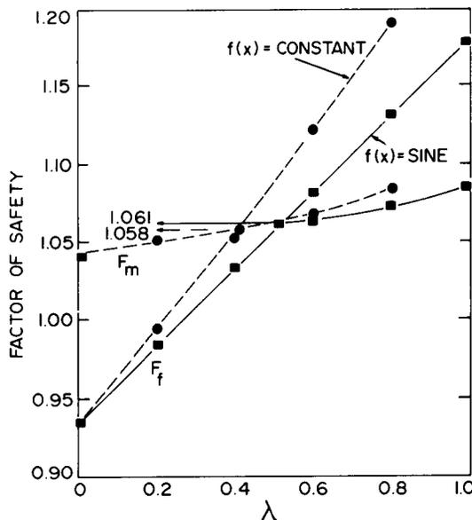
FIG. 7. Variation of the factor of safety with respect to moment and force equilibrium vs.  $\lambda$  for the Morgenstern-Price method. Soil properties:  $c'/\gamma h = 0.02$ ;  $\phi' = 40^\circ$ ;  $r_u = 0.5$ . Geometry: slope =  $26.5^\circ$ ; height = 100 ft (30 m).
