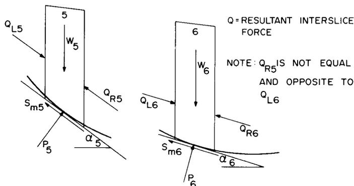
FIG. 2 Interslice forces for the ordinary method.
