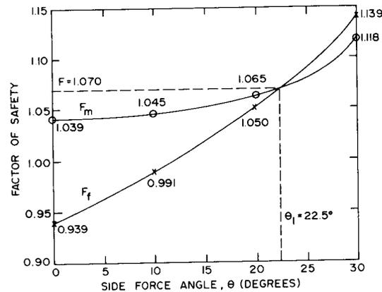
FIG. 3 Variation of the factor of safety with respect to moment and force equilibrium vs. the angle of the side forces. Soil properties:  $c'/\gamma h = 0.02$ ;  $\phi' = 40^\circ$ ;  $r_u = 0.5$ . Geometry: slope =  $26.5^\circ$ ; height = 100 ft (30 m).
