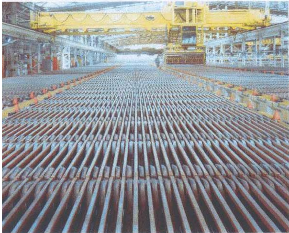
FIG. 1.7. Electrolytic Refinery Showing Cathodes Being Interweaved with Anodes in an Electrorefinery Cell (Photograph Courtesy Copper Refineries Pty., Townsville, Queensland).
