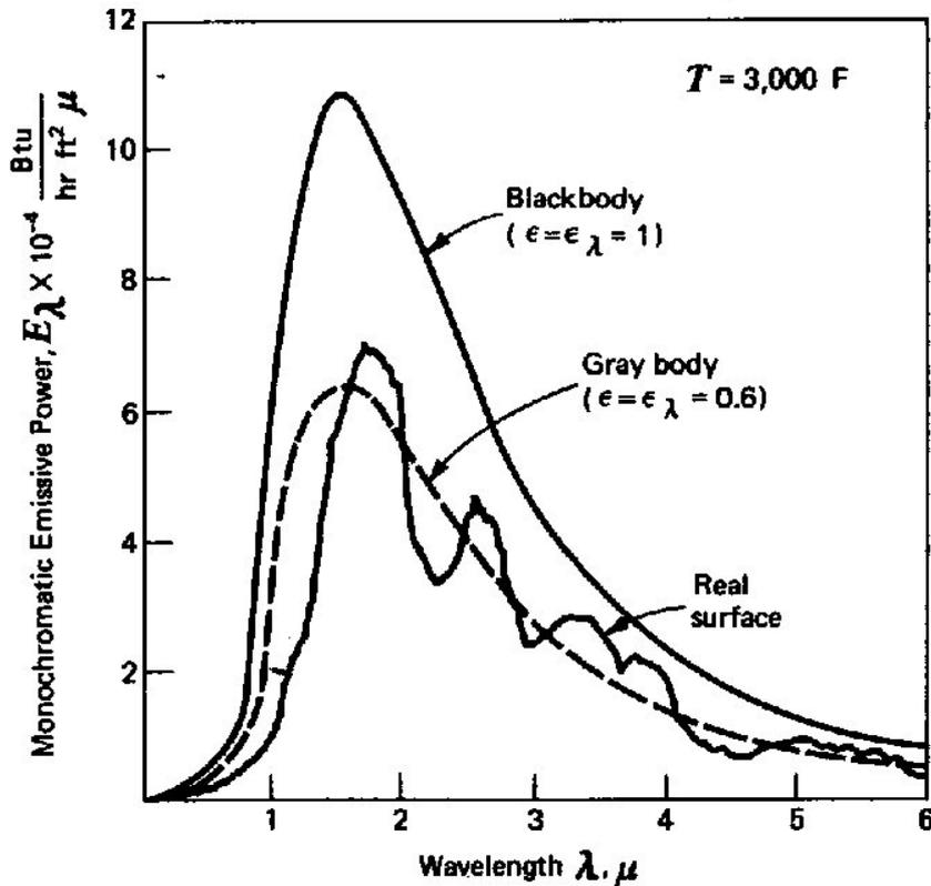
Fig. 5-9. Comparison of emissive power of black and gray bodies with that of a real surface.
