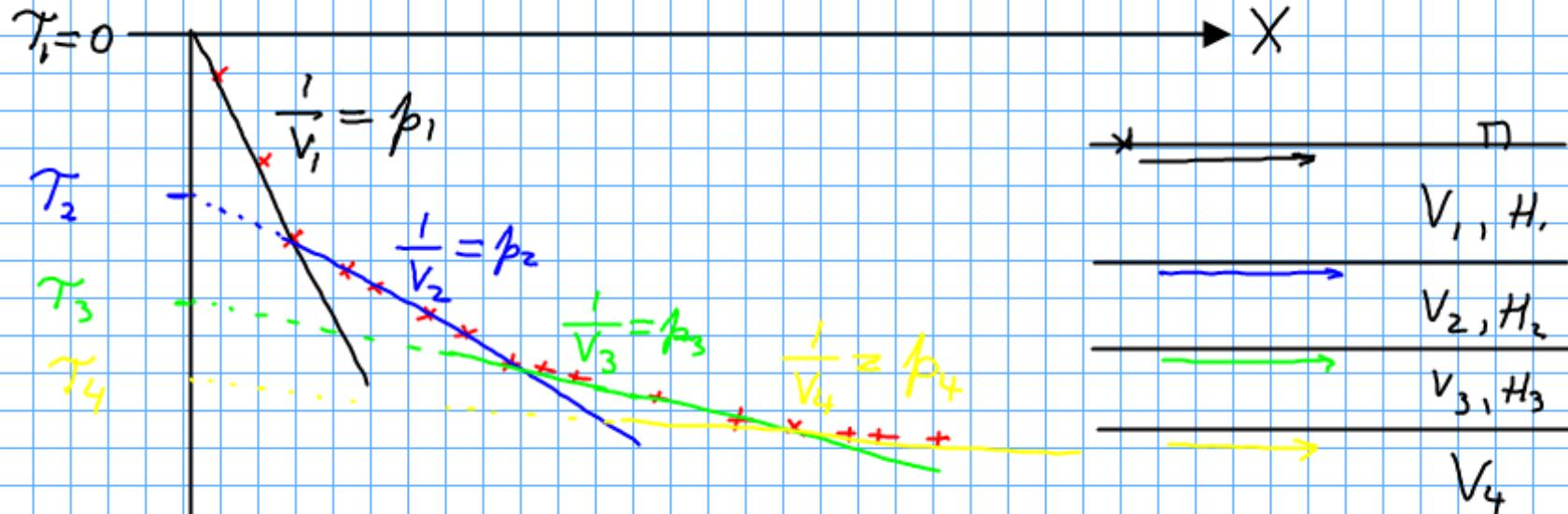
$$T_2 = 2H_1 \sqrt{\frac{1}{V_1^2} - \frac{1}{V_2^2}} = 2H_1 \sqrt{p_1^2 - p_2^2}$$
