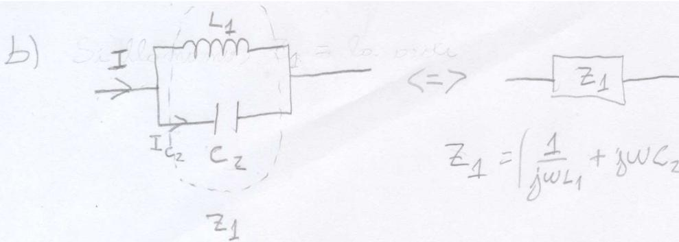
$$Z_1 = \left( \frac{1}{j\omega L_1} + j\omega C_2 \right)^{-1} = \frac{j\omega L_1}{1 - \omega^2 C_2 L_1}$$
