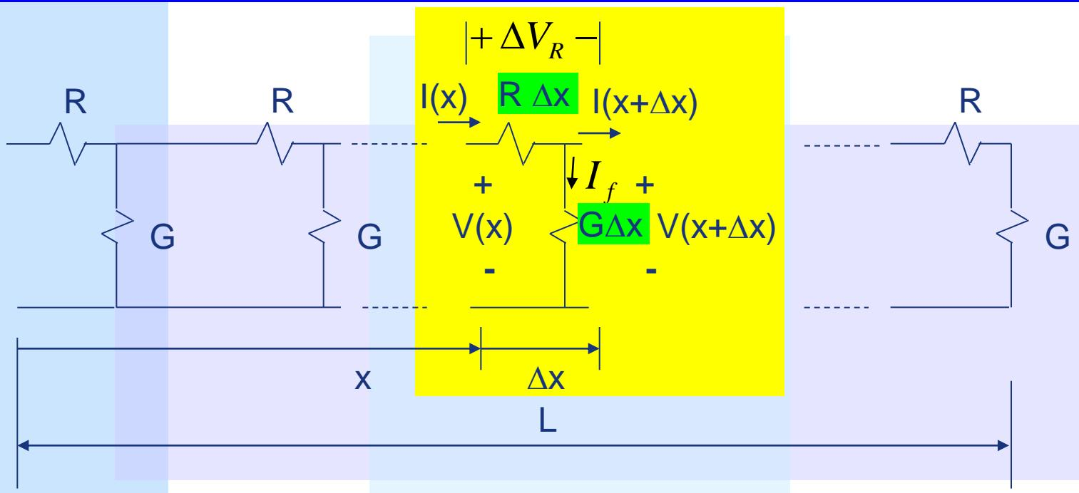
$$\text{LVK: } V(x) = \Delta V_R + V(x + \Delta x) \quad \Delta V_R = (R\Delta x)I(x)$$
