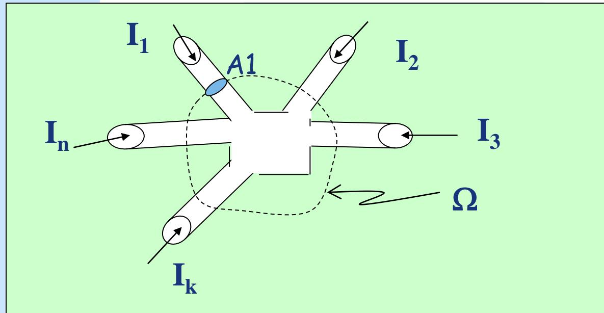
$$\frac{\partial \rho}{\partial t} = 0 \Rightarrow \nabla \cdot \vec{J} = 0 \quad \Rightarrow \iiint_{\Omega} \nabla \cdot \vec{J} dV = 0 \Rightarrow \iint_{S(\Omega)} \vec{J} \bullet d\vec{s} = 0$$
