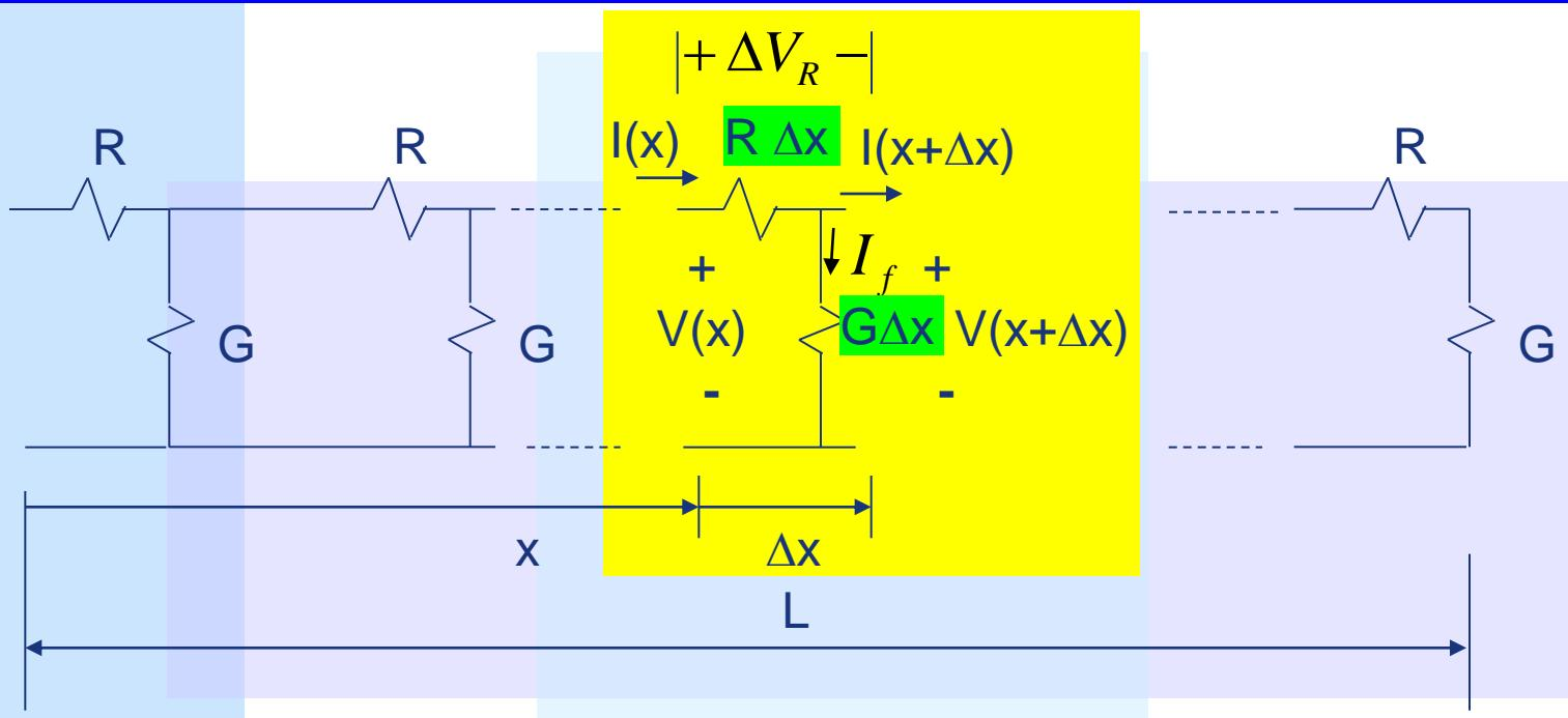
$$\frac{\partial^2 V(x)}{\partial x^2} = (RG)V(x) \rightarrow V(x) = Ce^{-x/\lambda} + De^{x/\lambda} \text{ con } \lambda^2 = RG$$
