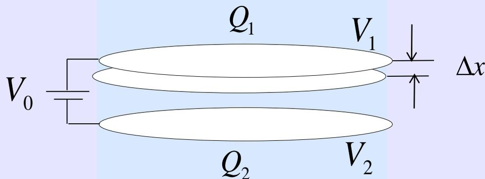
$$\Delta W = -\frac{1}{2} \sum V_i \Delta Q_i \Rightarrow \Delta W = -\frac{1}{2} (V_1 \Delta Q_1 + V_2 \Delta Q_2) \Rightarrow$$
