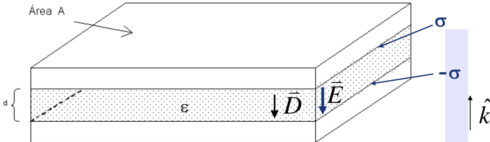
$$\vec{D} = -\sigma \hat{k} \Rightarrow \vec{E} = -\frac{\sigma}{\epsilon} \hat{k} \Rightarrow -\int_{-d}^0 \vec{E} \cdot d\vec{l} = V_{\sigma} - V_{-\sigma} \Rightarrow \overbrace{V_{\sigma} - V_{-\sigma}}^{\Delta V} = \frac{\sigma}{\epsilon} d$$
