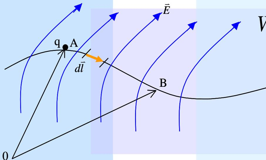
$$W = \int_A^B dW = -q \int_A^B \vec{E} \cdot d\vec{l} = q \underbrace{\int_B^A \vec{E} \cdot d\vec{l}}_{V_{BA}}$$
