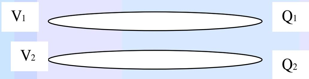
$$W = \frac{1}{2} \sum V_i Q_i \Rightarrow W = \frac{1}{2} (V_1 Q_1 + V_2 Q_2) \Rightarrow Q_2 = -Q_1 \Rightarrow W = \frac{1}{2} (V_1 - V_2) Q_1$$
