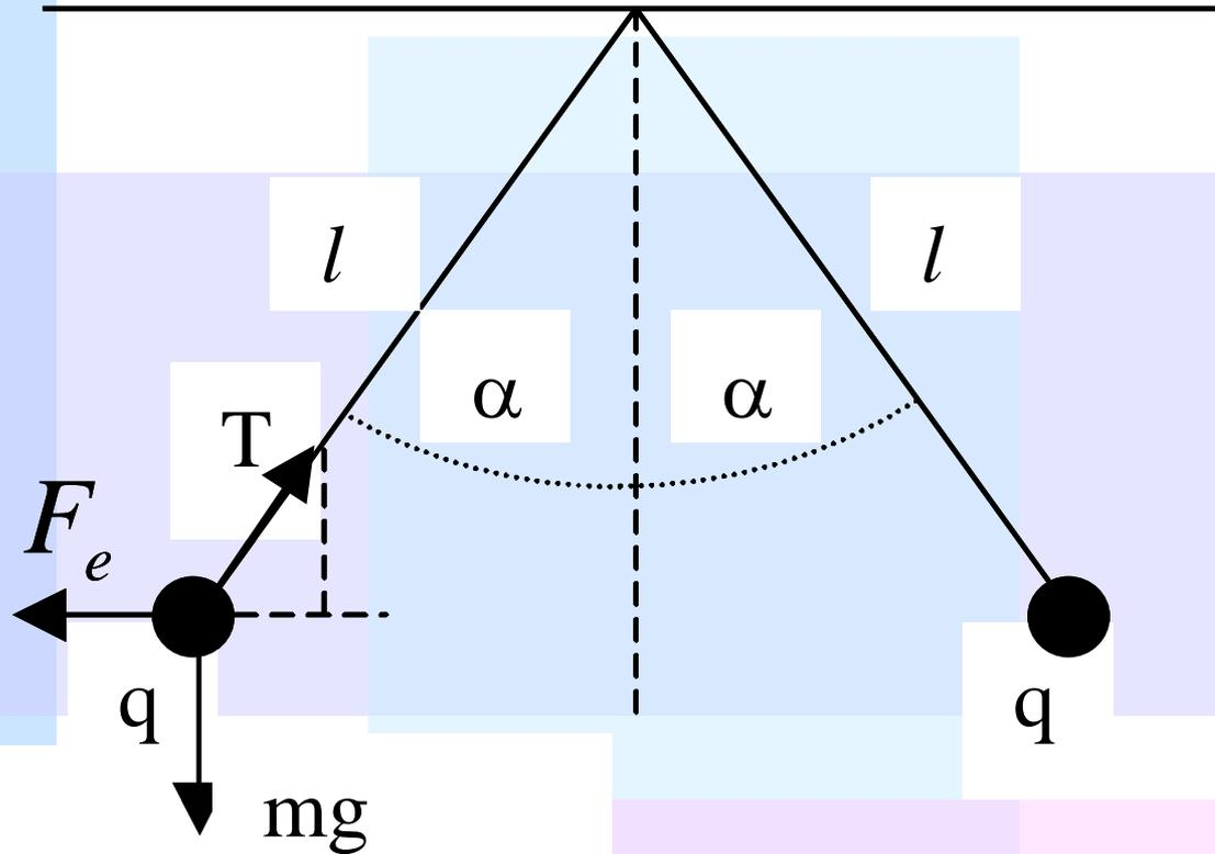
$$\left. \begin{array}{l} F_e = T \sin \alpha \\ mg = T \cos \alpha \end{array} \right\} \Rightarrow \frac{F_e}{mg} = \frac{\sin \alpha}{\cos \alpha}$$
