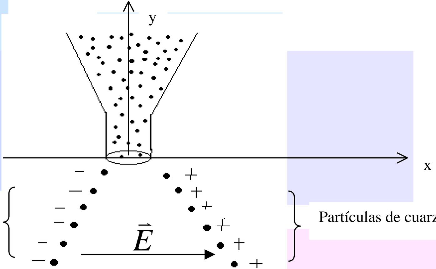
$$\vec{F} = m \cdot \vec{a} \quad \vec{F} = F_e \hat{x} + \vec{F}_g \hat{y} \quad \Rightarrow q \cdot \vec{E} = m \frac{d^2 x}{dt^2} \quad -mg = m \frac{d^2 y}{dt^2}$$
