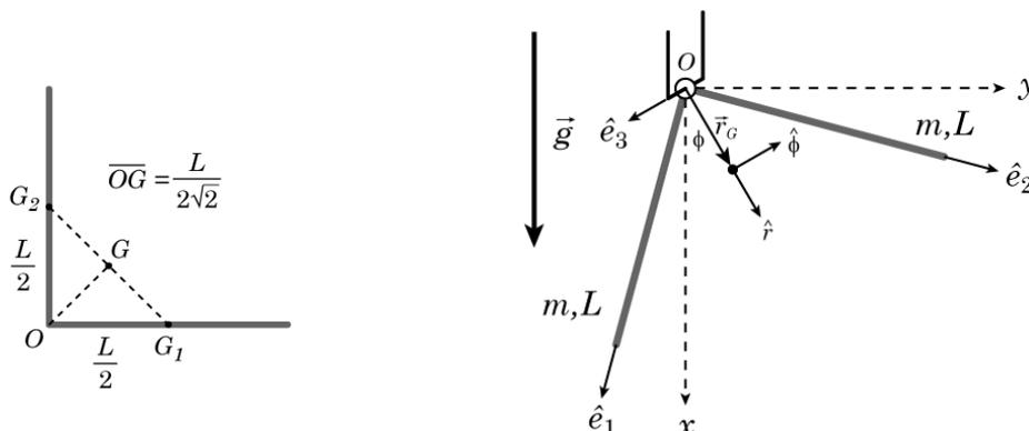
$$\vec{r}_G = \frac{1}{2\sqrt{2}}L\hat{r}, \quad \vec{v}_G = \frac{1}{2\sqrt{2}}L\dot{\phi}\hat{\phi}, \quad \vec{a}_G = \frac{1}{2\sqrt{2}}L(-\dot{\phi}^2\hat{r} + \ddot{\phi}\hat{\phi})$$
