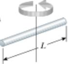
Long thin rod with rotation axis through end
