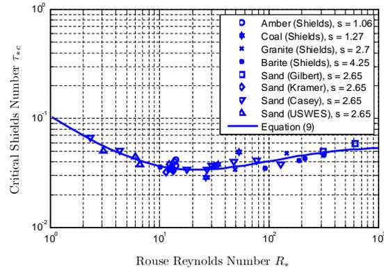
Fig. 3. Shields-Rouse diagram for sediment incipient motion
