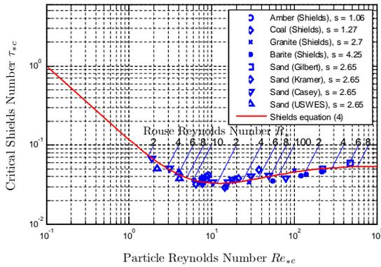
Fig. 2. Shields diagram for sediment incipient motion [Data source: Table 3 in Buffington (1999)]
