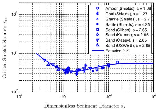
Fig. 4. Shields-Rouse equation in terms of  $d_*$
