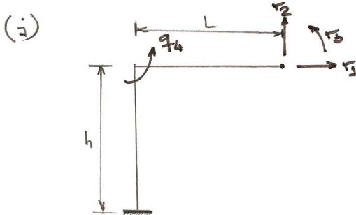
$$[K_1] = EI \begin{bmatrix} \frac{1}{12/h^3} & \frac{1}{2} & \frac{1}{2} & \frac{q_4}{6/h^2} \\ 0 & \frac{1}{12/L^3} & -6/L^2 & -6/L^2 \\ 0 & -6/L^2 & 4/L & 2/L \\ 6/h^2 & -6/L^2 & 2/L & 4/h + 4/L \end{bmatrix} \quad (4)$$
