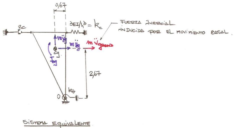
DE LA FIGURA,  $m = \frac{W}{g} = \frac{2000}{9,8} = 204,1 \left[ \frac{\text{kg} \cdot \text{s}^2}{\text{m}} \right]$  (1a)
