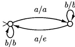
$a/w$ , which means “if the input symbol is  $a$ , follow this arrow and emit output  $w$ ”. For example, the deterministic finite-state transducer over  $\{a, b\}$  shown above transmits all  $b$ 's in the input string but omits every other  $a$ .
