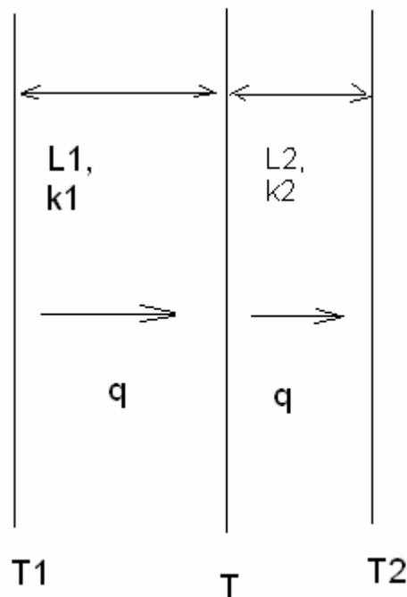
$$q_1 = \frac{k_1(T_1 - T)}{L_1} \quad q_2 = \frac{k_2(T - T_2)}{L_2}$$
