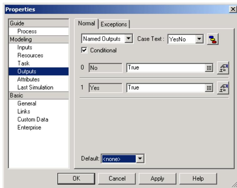
A transaction follows a directed connector line or lines out of an activity to the inputs of the next activity. The Normal tab, used on most activities, defines how transactions follow lines. The Exceptions tab specifies any special outputs.
