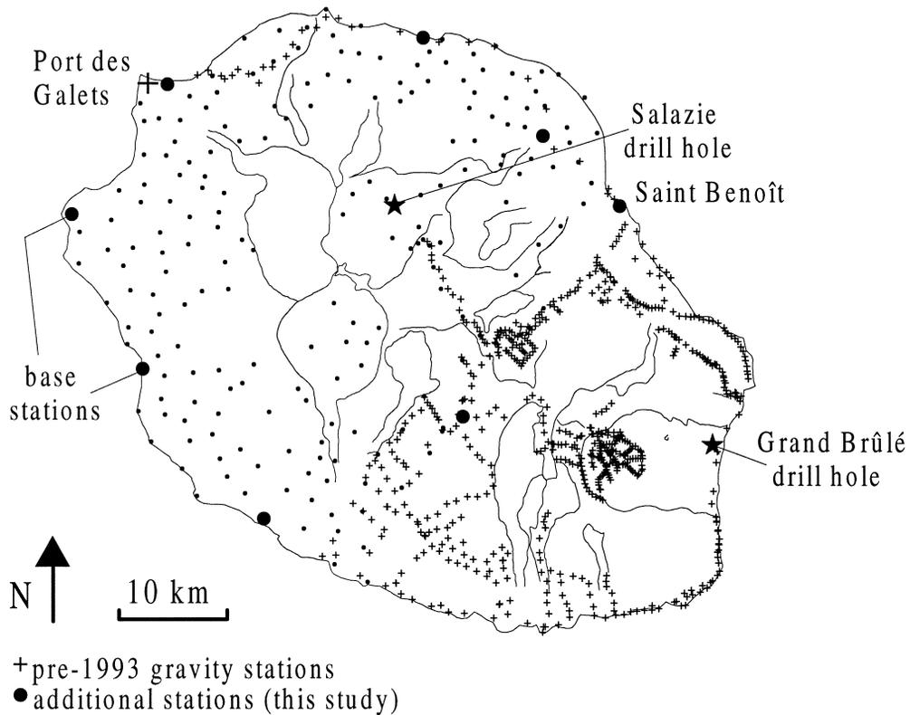
Fig. 2. Distribution of the available gravity data acquired on land before 1993 (crosses) and of the new gravity stations set up in 1993 on the western side of the island (full circles).
