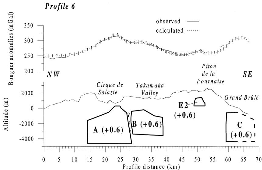
Fig. 7. 2.5D model on the NW–SE profile 6 shown in Fig. 4. The observed curve (gravity field obtained for a correction density of  $2.7 \times 10^3 \text{ kg/m}^3$ ) is drawn only in areas where data have been acquired. Density contrasts are in  $10^3 \text{ kg/m}^3$  and errors on calculated gravity field are rms errors. Eastern boundaries of body C are drawn as dashed lines as they are based on results from previous detailed gravity surveys (see text).
