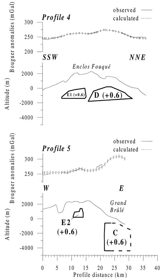
Fig. 6. 2.5D models on profiles 4 and 5 (shown in Fig. 4) on the eastern side of the island. The observed curve (gravity field obtained for a correction density of  $2.7 \times 10^3 \text{ kg/m}^3$ ) is drawn only in areas where data have been acquired. Density contrasts are in  $10^3 \text{ kg/m}^3$  and errors on calculated gravity field are rms errors. Eastern boundaries of body C are drawn as dashed lines as they are based on results from previous detailed gravity surveys (see text).
