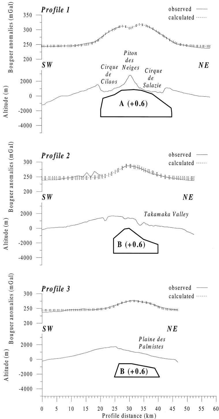
Fig. 5. 2.5D models on SW–NE profiles 1, 2 and 3 (shown in Fig. 4) on the western side of the island. The observed curve (gravity field obtained for a correction density of  $2.7 \times 10^3 \text{ kg/m}^3$ ) is drawn only in areas where data have been acquired. Density contrasts are in  $10^3 \text{ kg/m}^3$  and errors on calculated gravity field are rms errors.
