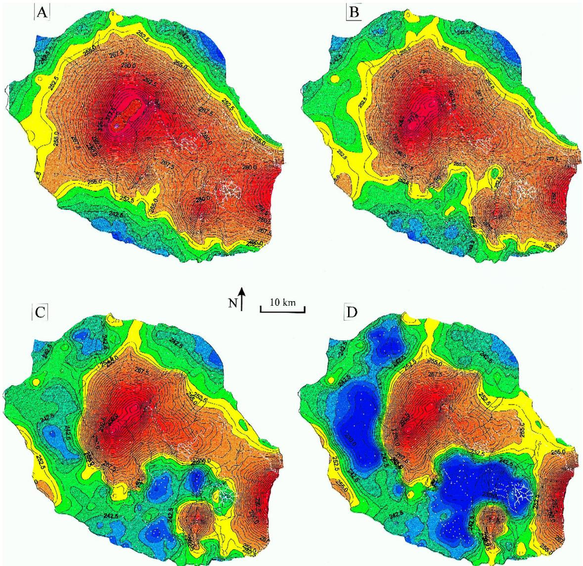
Fig. 3. Bouguer anomaly maps of Réunion Island computed with all available data. The density corrections are  $2.5 \times 10^3 \text{ kg/m}^3$  (A),  $2.7 \times 10^3 \text{ kg/m}^3$  (B),  $2.9 \times 10^3 \text{ kg/m}^3$  (C) and  $3.1 \times 10^3 \text{ kg/m}^3$  (D). Contour interval is 2.5 mGal.
