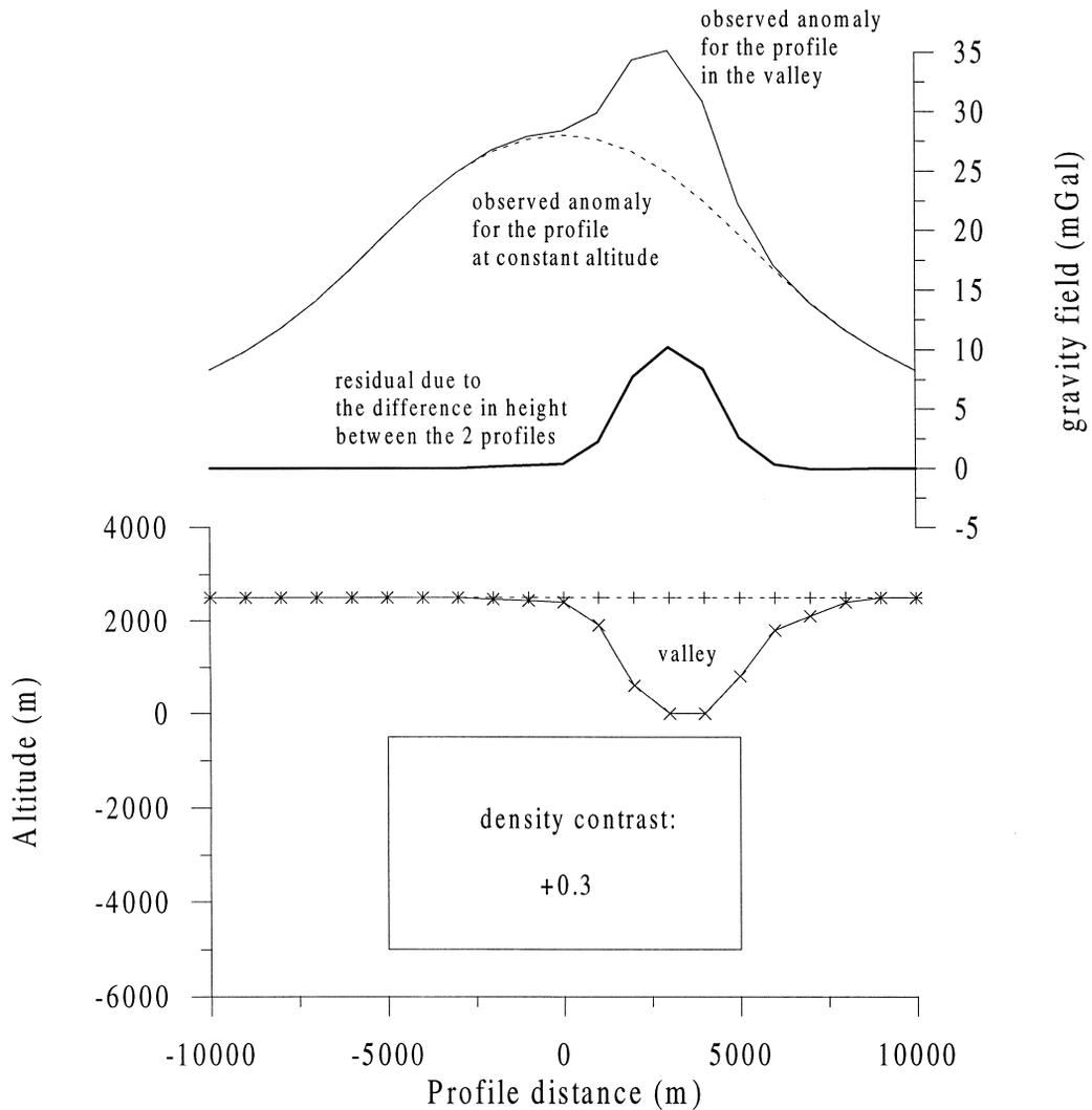
Fig. 8. Theoretical model showing the relation between the anomaly pattern and the variable height of gravity stations when a density contrast exists at shallow depth.
