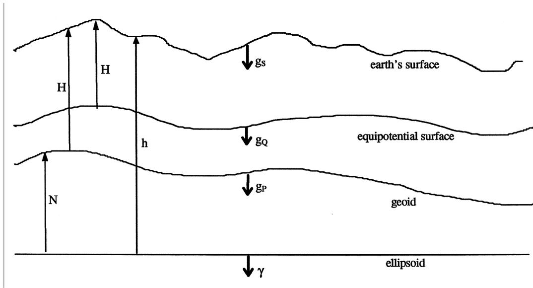
Figure 1. Surface gravity ( $g_s$ ), geoidal gravity ( $g_P$ ), normal gravity ( $\gamma$ ) and gravity on arbitrary equipotential surface ( $g_Q$ ).  $N$  is geoid-ellipsoid separation,  $H$  is height relative to geoid or any other equipotential surface, and  $h$  is ellipsoidal height.
