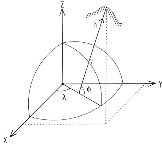
Figure 2. Geometrical relationship between Cartesian coordinates ( $X, Y, Z$ ) and ellipsoidal coordinates ( $\phi, \lambda, h$ ).
