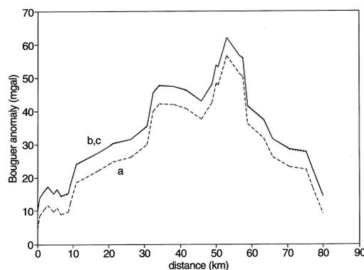
Figure 3. Simple Bouguer anomalies derived from (a) WGS84 ellipsoidal coordinates alone (dashed line), (b) AGD84 geodetic coordinates and AHD heights (dotted line), and (c) WGS84 geodetic coordinates and GPS-geoid derived AHD heights (solid line) (units in mgal).
