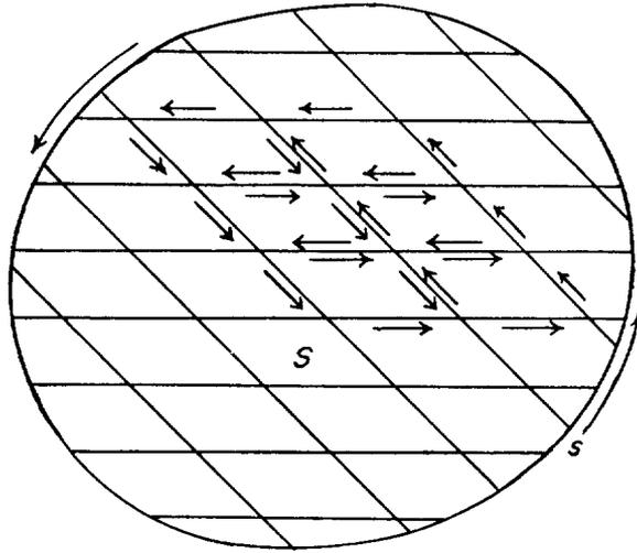
FIG. 5. Conversion of surface integral to line integral.
