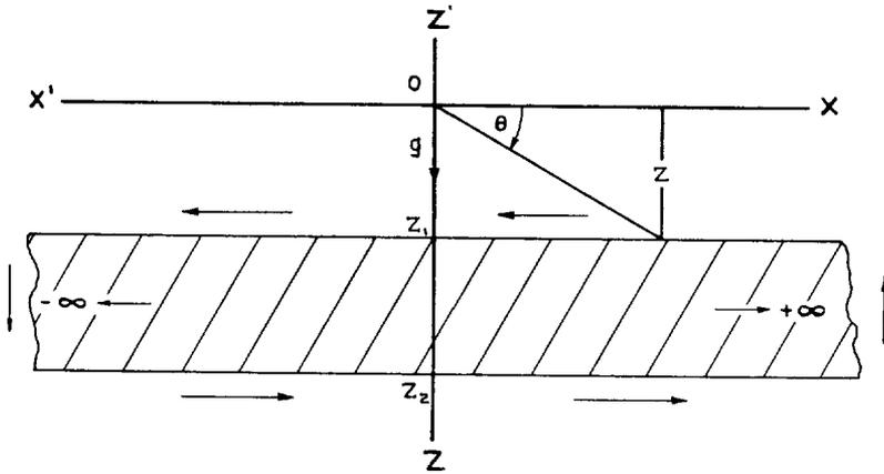
FIG. 6. Calculation of attraction of infinite plate by means of line integrals.
