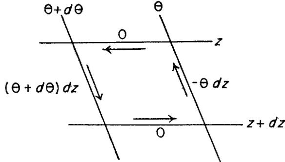
FIG. 4. Line integral about a  $d\theta dz$ -solenoid.
