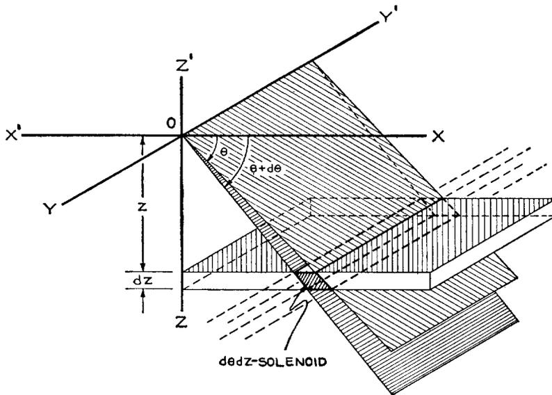
FIG. 2. Illustration of  $d\theta dz$ -solenoid.
