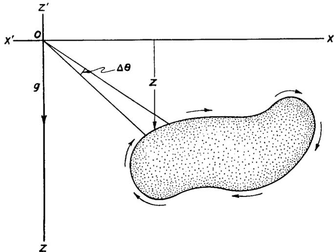
FIG. 8. Geometrical elements involved in evaluating  $\oint z d\theta$ .
