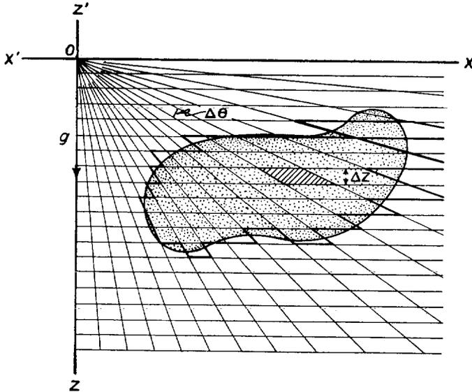
Fig. 3. Calculation of gravitational attraction by areal integration of  $d\theta dz$ -solenoids.
