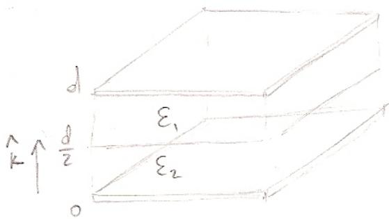
$$\vec{D}(z) = \begin{cases} 0 & \text{si } d < z \\ \sigma_0 \hat{k} & \text{si } 0 < z < d \\ 0 & \text{si } z < 0 \end{cases}$$
