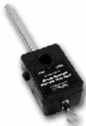
The Dual-Range Force Sensor is a general-purpose device for measuring pushing and pulling forces. It can be used as a replacement for a hand-held spring scale or mounted on a ring stand. It can also be mounted on a dynamics cart to study collisions. Forces as small as 0.01 newtons and as large as 50 newtons can be measured. The Dual-Range Force Sensor can be used for a variety of experiments, including
