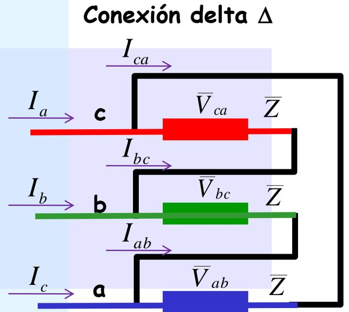
$$V = V_{\Delta} \quad I = \sqrt{3} I_{\Delta}$$
