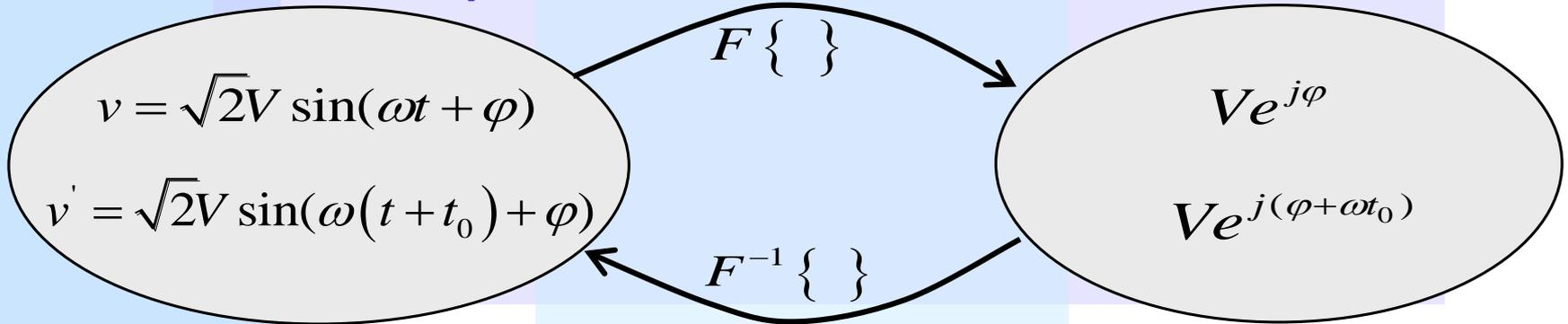
$$F \left\{ \sqrt{2}V \text{sen}(\omega t + \varphi) \right\} = Ve^{j\varphi}$$
