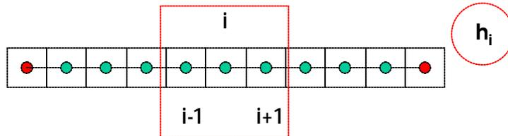
$$\frac{\partial^2 h}{\partial x^2} \Big|_i = \frac{\partial}{\partial x} \left( \frac{\partial h}{\partial x} \right) \Big|_i \cong \frac{\frac{\partial h}{\partial x} \Big|_i - \frac{\partial h}{\partial x} \Big|_{i-1}}{\Delta x} = \frac{\left( \frac{h_{i+1} - h_i}{\Delta x} \right) - \left( \frac{h_i - h_{i-1}}{\Delta x} \right)}{\Delta x}$$
