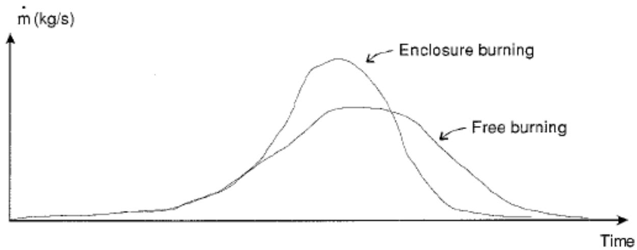
FIGURE 3.2 The enclosure effect on mass loss rate.
