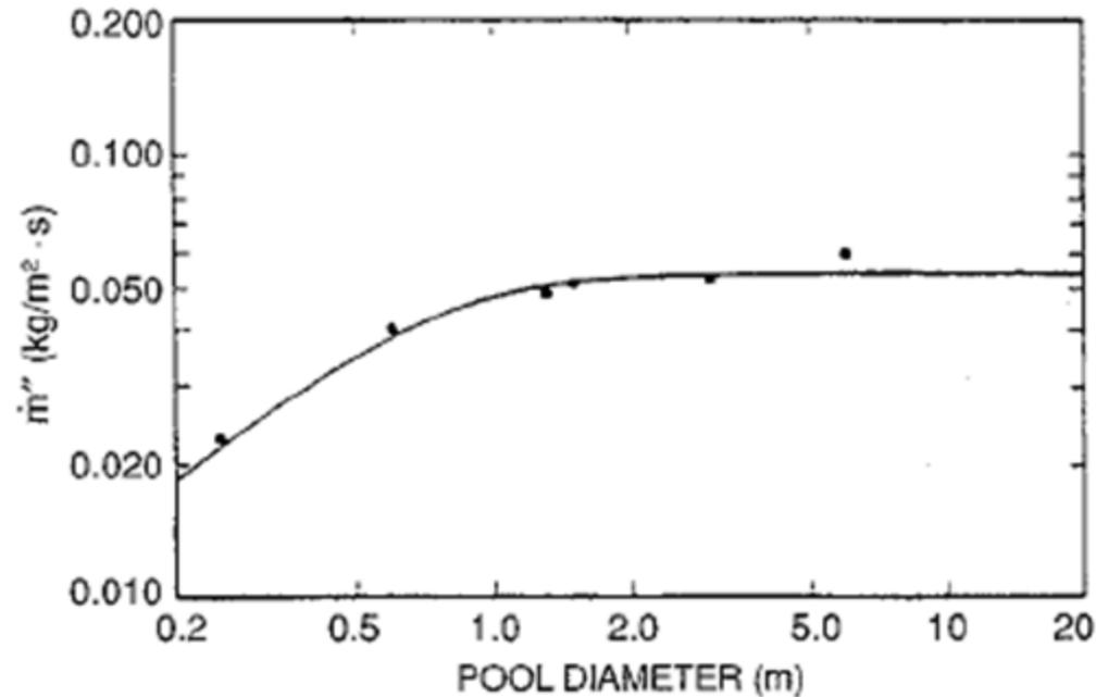
FIGURE 3.5 Mass loss rate for gasoline pools of various diameters. (From Babrauskas<sup>1</sup>. With permission.)
