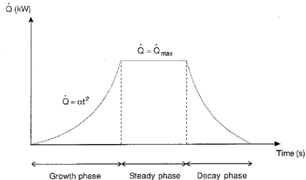
**FIGURE 3.15** A simple design fire curve.
