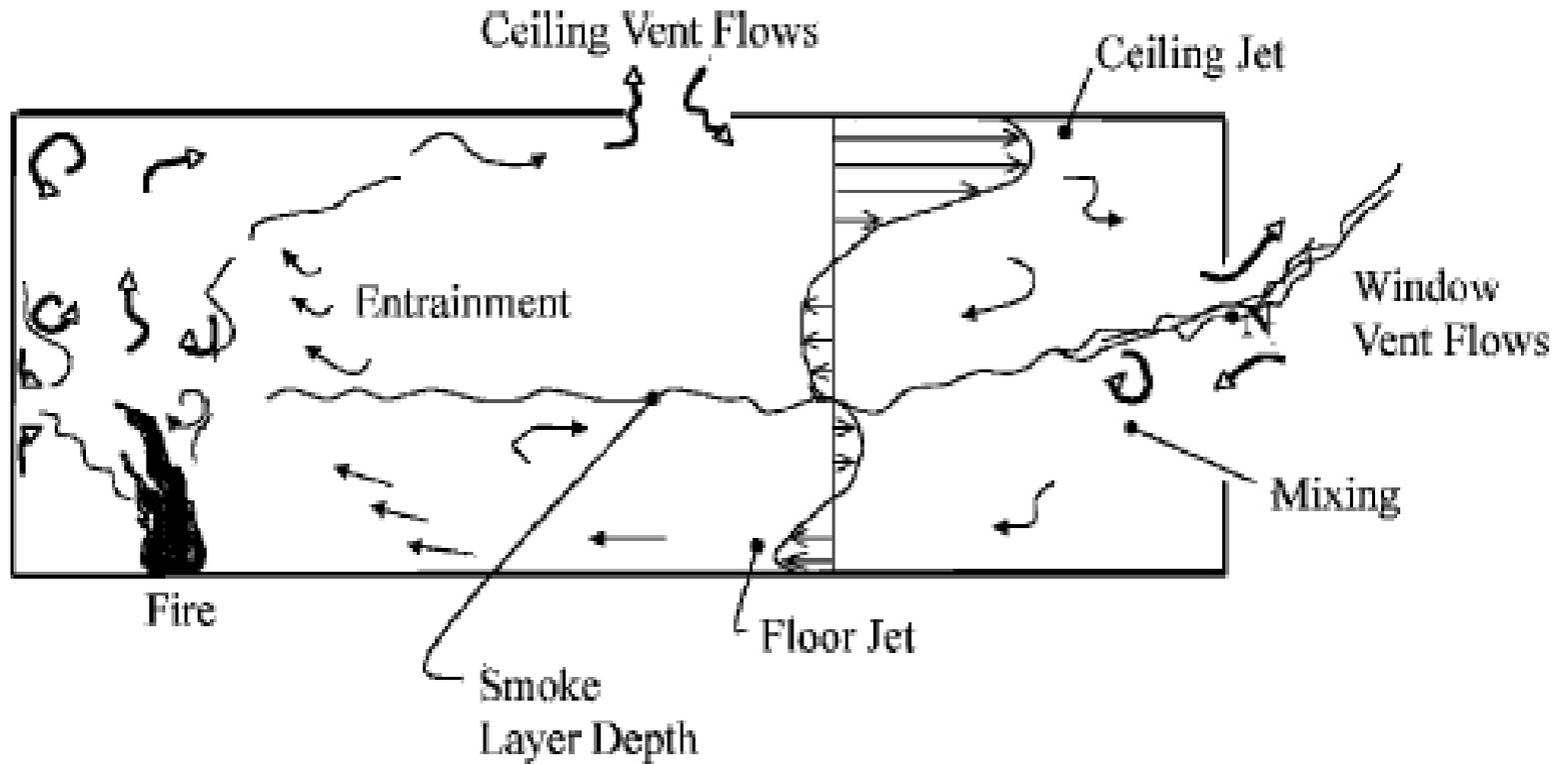
Figure 11.3 Flow pattern in a compartment fire
