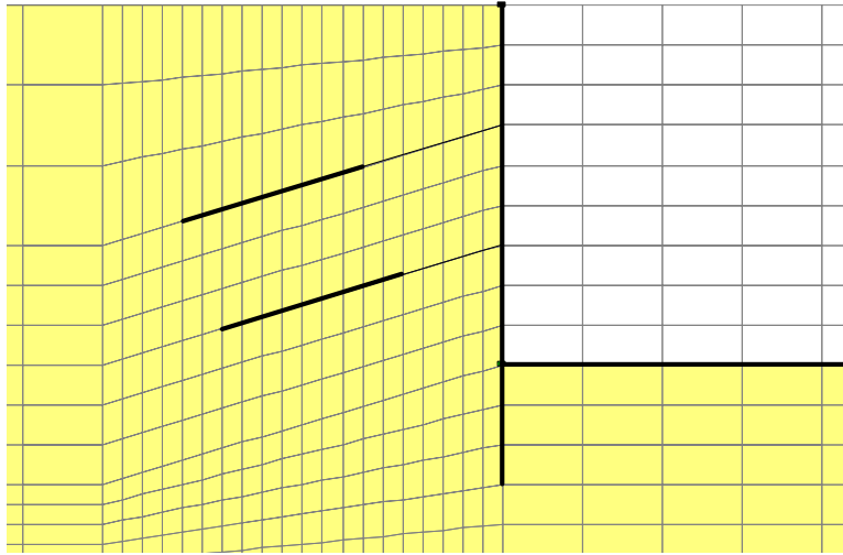
Figure 8-31 A sheet pile wall with pre-stressed tie-back anchors
