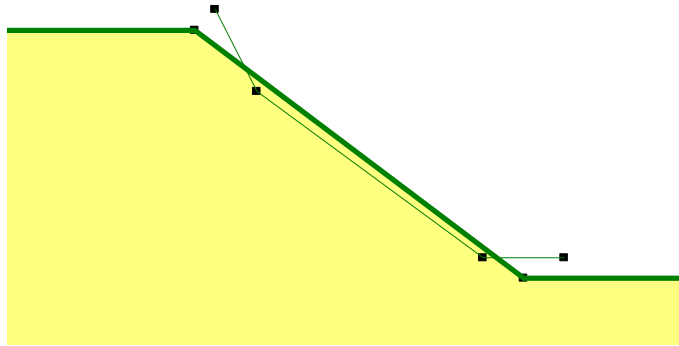
Figure 4-51 Slip surface with thickness less than specified minimum
