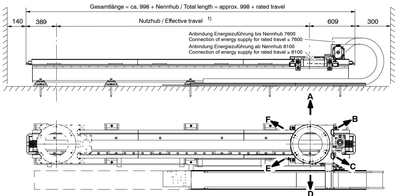
A, B, C, D, E, F = Robotermontagevarianten / Robot mounting variants
