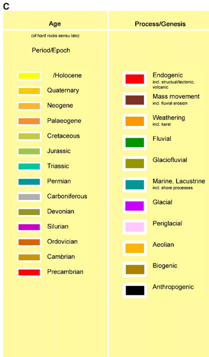
Fig. 1. The new legend. This system combines lines, hatching, symbols and letters/figures with colours. The flexible legend makes it possible to include a wider range of geomorphological parameters than previous mapping systems.
