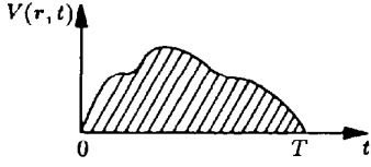
Fig. 11.2. General form of a perturbation in the time period 0 \leq t \leq T . Such a perturbation can be caused, for example, by an external field, which is switched on during this period, or by a particle that is passing by. In the latter case, T is a measure of the collision (interaction) time
