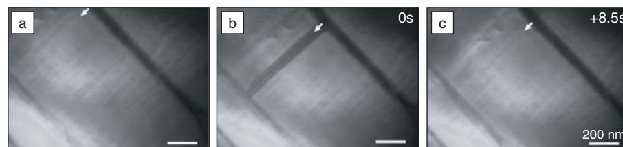
Figure 13. Video frame images showing the glide of partial dislocations. (a) Before and (b) after the glide of a leading partial dislocation that was emitted from the twin aa' (the white arrow). The stacking fault was left behind the partial dislocation. (c) A few seconds after the first partial (in this case, 8.5 s), the trailing partial was emitted and swept out the stacking fault. Then, the partials recombined to a perfect dislocation which cross-slipped into the twin bb' . 102 All three micrographs were taken at same scale. (Reproduced with permission from Oh et al, Acta Mater. 55 :5558 © 2007 Elsevier)
