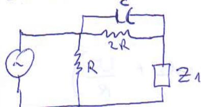
$$Z_1 = j\omega L // 2R \xrightarrow{\text{"suma en paralelo"}} \left( \frac{1}{j\omega L} + \frac{1}{2R} \right)^{-1} = \frac{j\omega 2RL}{j\omega L + 2R} = \frac{2R}{1 + \frac{j\omega L}{2R}}$$
