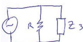
$$Z_3 = Z_1 + Z_2 \xrightarrow{\text{"suma en serie"}} = \frac{2R}{1 + \frac{j\omega L}{2R}} + \frac{2R}{1 + j\omega 2RC} = \frac{2R(1 + j\omega 2RC + 1 + \frac{j\omega L}{2R})}{(1 + \frac{j\omega L}{2R})(1 + j\omega 2RC)}$$
