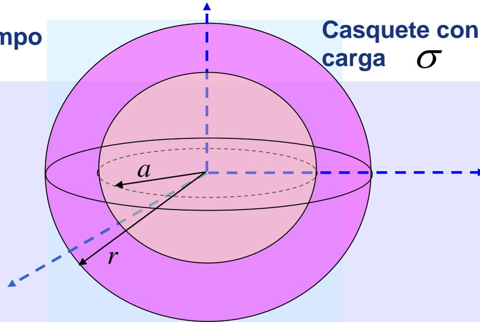
$$V(\vec{r}) = \frac{\sigma a^2}{\epsilon_0 r} \Big|_{r_0}^r + V_{ref}(r = r_0) = \frac{\sigma a^2}{\epsilon_0 r} - \frac{\sigma a}{\epsilon_0 a} + V_{ref}(r = r_0)$$
