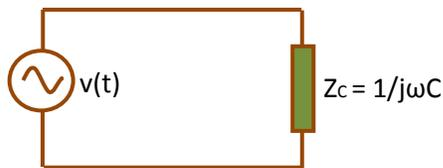
$$v(t) = V_m \sin(\omega t) \rightarrow i_c(t) = C \frac{dv(t)}{dt} = \omega C V_m \cos(\omega t)$$
