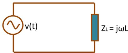
$$v(t) = V_m \sin(\omega t) \rightarrow i_L(t) = \int v(t) dt = -\frac{V_m}{\omega L} \cos(\omega t)$$
