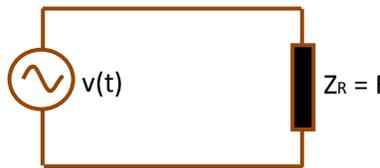
$$v(t) = V_m \sin(\omega t) \rightarrow i_R(t) = \frac{v(t)}{R} = \frac{V_m \sin(\omega t)}{R} \rightarrow \varphi = 0$$
