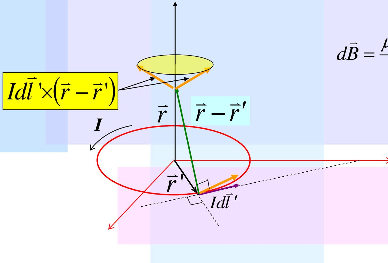
$$d\vec{B} = \frac{\mu_0 I d\vec{l}' \times (\vec{r} - \vec{r}')}{4\pi \|\vec{r} - \vec{r}'\|^3}$$
