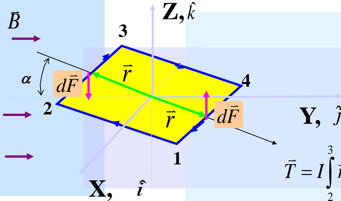
$$\vec{T} = I \int_2^3 \vec{r} \times dx \hat{i} \times \vec{B} + I \int_4^1 \vec{r} \times dx \hat{i} \times \vec{B}$$
