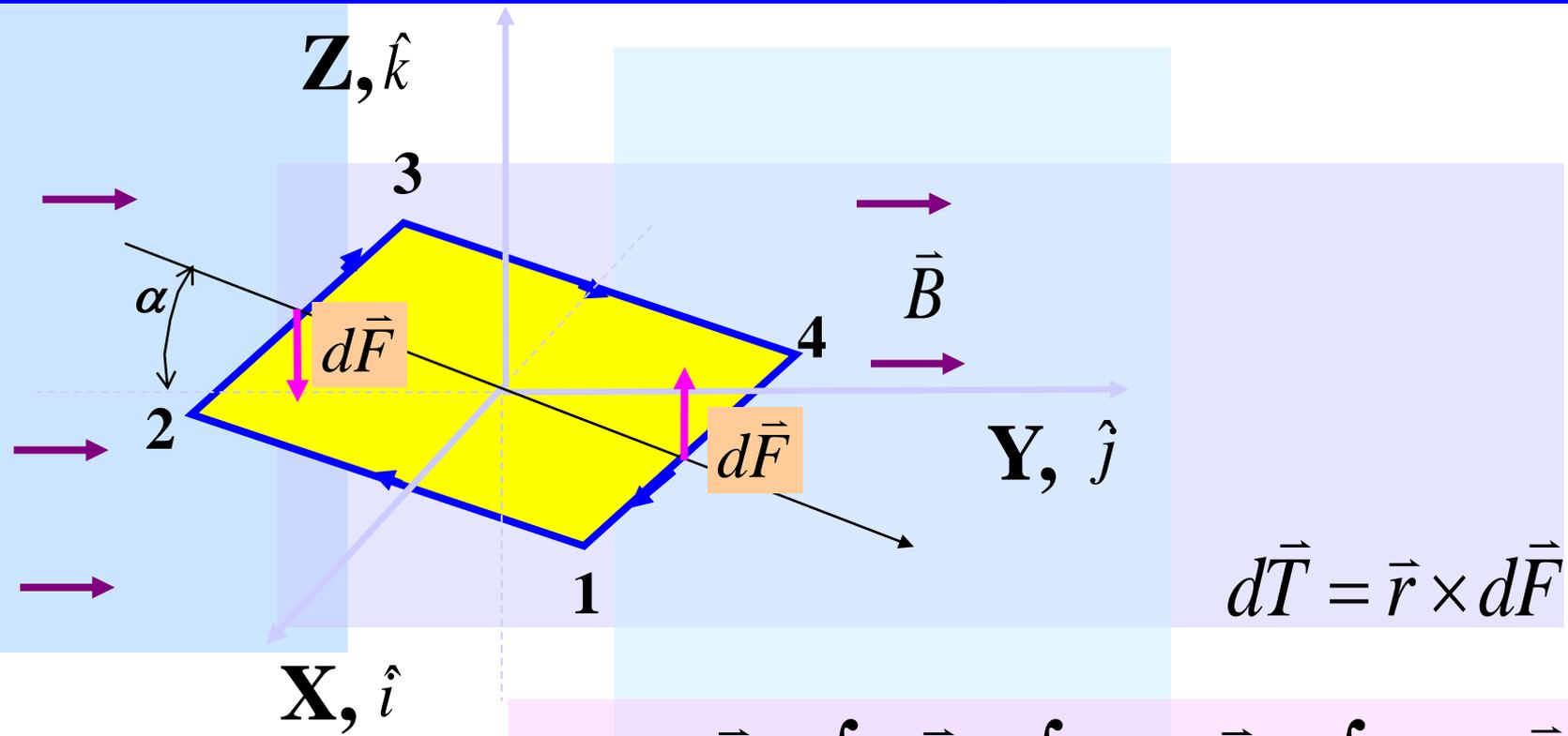
$$\vec{T} = \oint_c d\vec{T} = \oint_c \vec{r} \times d\vec{F} = \oint_c \vec{r} \times id\vec{l} \times \vec{B}$$
