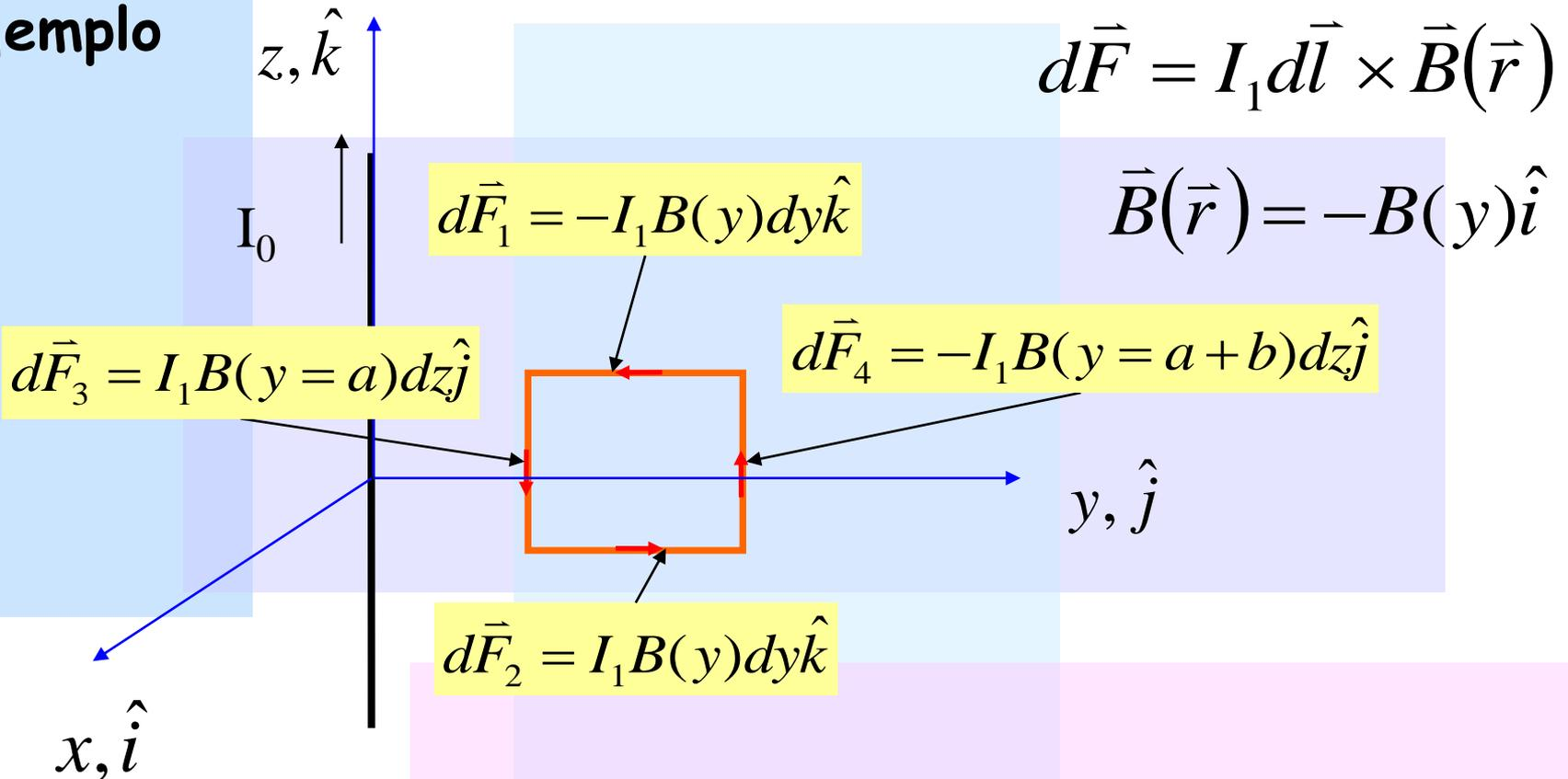
$$\vec{F} = \oint_{\Gamma} d\vec{F} = \int_{z=b/2}^{z=-b/2} \frac{\mu_0 I_1 I_0 \hat{j}}{2\pi a} dz - \int_{z=-b/2}^{z=b/2} \frac{\mu_0 I_1 I_0 \hat{j}}{2\pi(a+b)} dz = \frac{\mu_0 I_1 I_0 b^2}{2\pi(a+b)} \hat{j}$$
