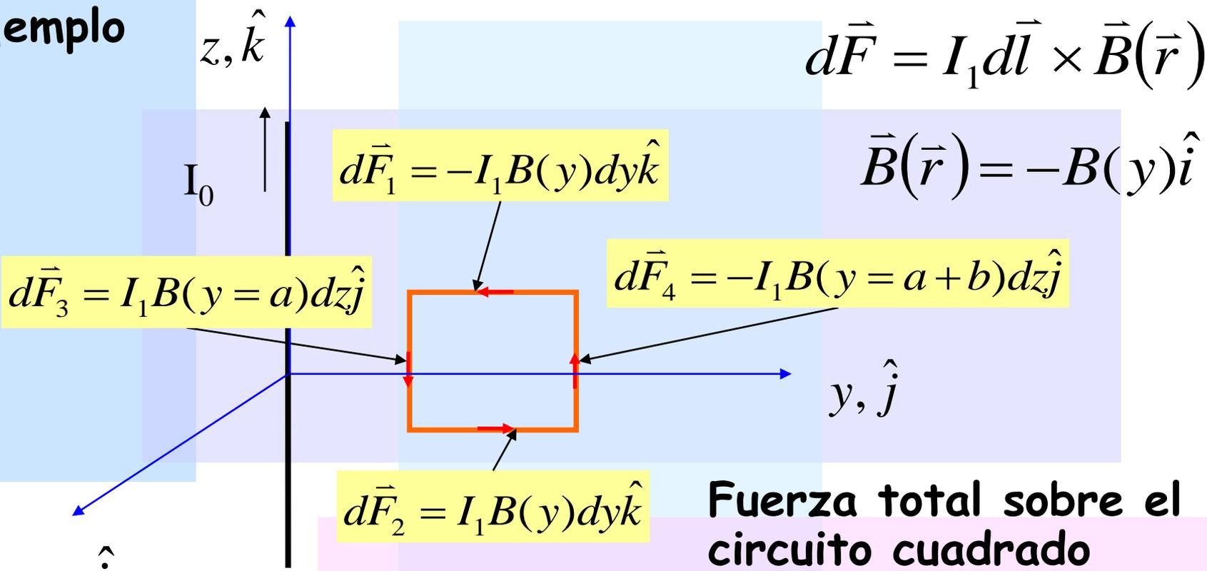
$$\therefore \vec{F} = \oint_{\Gamma} d\vec{F} = \int_{y=a+b}^{y=a} d\vec{F}_1 + \int_{z=b/2}^{z=-b/2} d\vec{F}_3 + \int_{y=a}^{y=a+b} d\vec{F}_2 + \int_{z=-b/2}^{z=b/2} d\vec{F}_4$$
