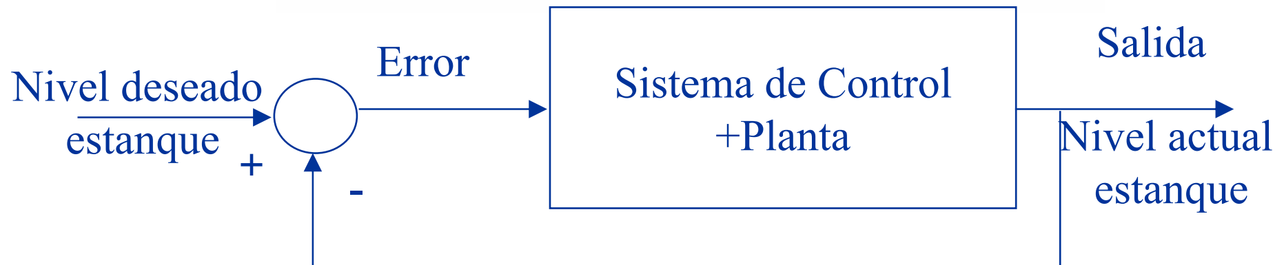
Figure 1.7 Automatic tank-level control system.
