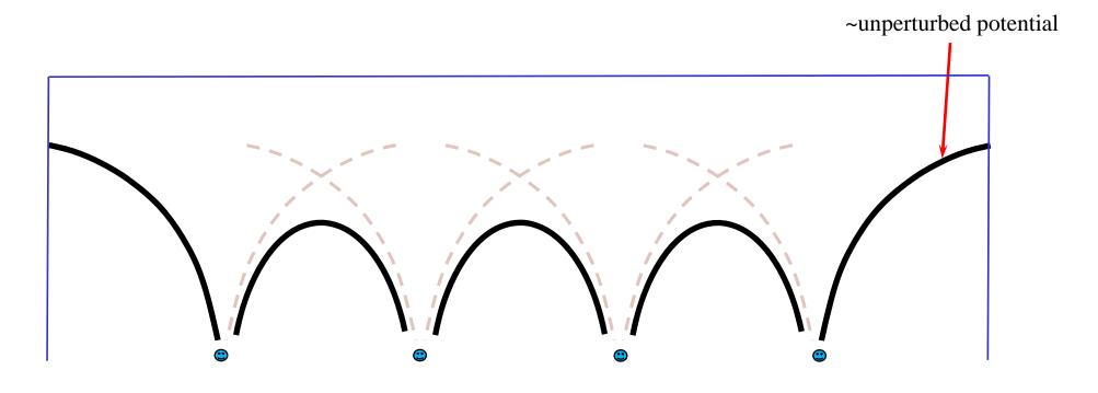
The potential barrier confines the electrons inside the faces of the conductor. Therefore we can model a conductor as unbound or free electrons confined to a potential box.
